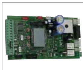
USER 1-24V DG control unit programmable with LED display and integrated warning light
