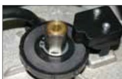
Mechanical twin-disc clutch (only for SATURN OIL)
