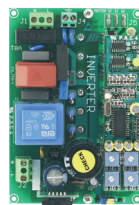
INVERTER Code ACG9201 Optional, to increase speed up to 0,28 m/s
