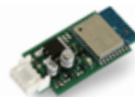
P-250T-WIFI Device for Wi-Fi connection 2,4 GHz to allow the smartphone to remotely control and program the control units via TauApp
