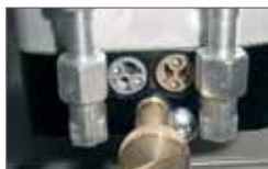
By pass valves for the force adjustment
