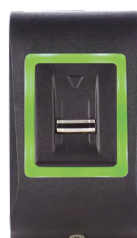
Green LED Access Granted
