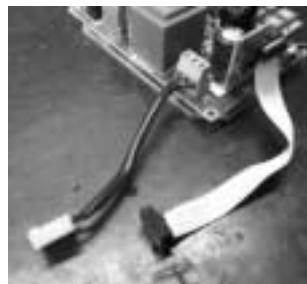
The inverter is supplied with power and logic connection cables for the KS card.
