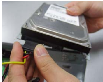
<Connecting power cable>
